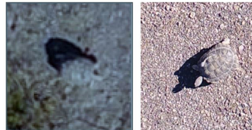
Drone imagery at 1cm pixel size vs. 0.5 cm pixel size. With the 0.5 pixel size being easier to detect from drone imagery.
